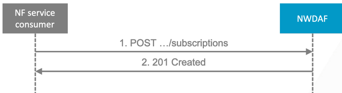
Figure 2 – An NF service consumer subscribes to NWDAF notifications
